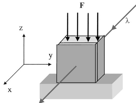
Fig. 1. Geometry used for the tensor calculation of changes in refractive index and mechanical thickness when the filter is loaded with a uniform uniaxial force  $F$ .
