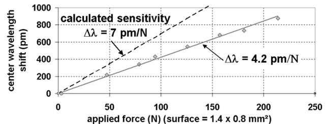
Fig. 2. Center wavelength shift: experimental data, solid line; simulated data, dashed line.
