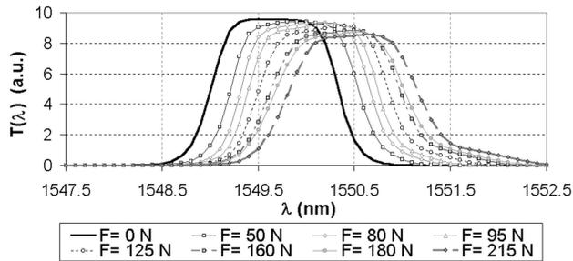
Fig. 3. Experimental transmittance curves for several cases of uniform loading.
